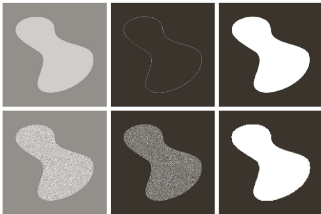
FIGURE 10.1 (a) Image containing a region of constant intensity. (b) Image showing the boundary of the inner region, obtained from intensity discontinuities. (c) Result of segmenting the image into two regions. (d) Image containing a textured region. (e) Result of edge computations. Note the large number of small edges that are connected to the original boundary, making it difficult to find a unique boundary using only edge information. (f) Result of segmentation based on region properties.
